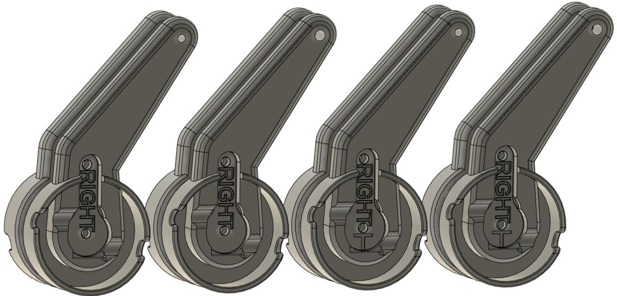
NOTE: I've updated this pack to contain both stock thickness arms and arms that are reduced by 0.5mm (some servo splines are a little farther out and this can cause the pitch arms to rub together more than desired) as well as arms that have 3mm and 4mm holes, if you find yourself using 3mm ID rod ends.
