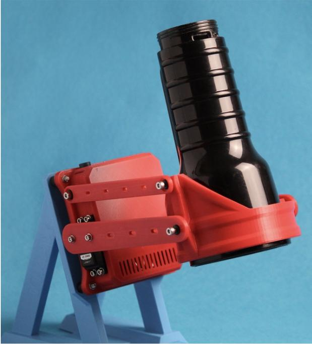
The **Open-source Stroker Robot, 2-axis** (OSR2) is a **Multi-Axis Stroker Robot** (MAxSR) designed to hold and move a standard [Fleshlight](#) or similar toy with 2-4 degrees of freedom.
